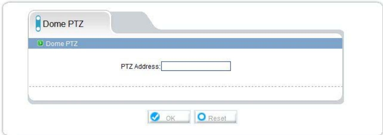
The motorized cameras speed dome RH series are equipped with an RS485 port that allows to control the movements with a keyboard for speed dome with Pelco P / D protocol. In this window it is possible to insert the RS485 address of the camera by typing on the keyboard to be able to be controlled. The communication data is then set in the section EXTERNAL DEVICE.
