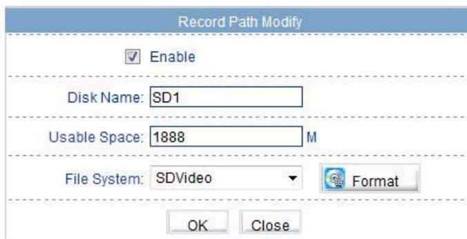
Click FORMAT and wait for the formatting is complete. There are 2 modes of file system for formatting: SD Video and EXT3. For practical purposes the two file systems are equivalent: SD Video is a proprietary file system and EXT3 file system is used by GNU / Linux systems.
