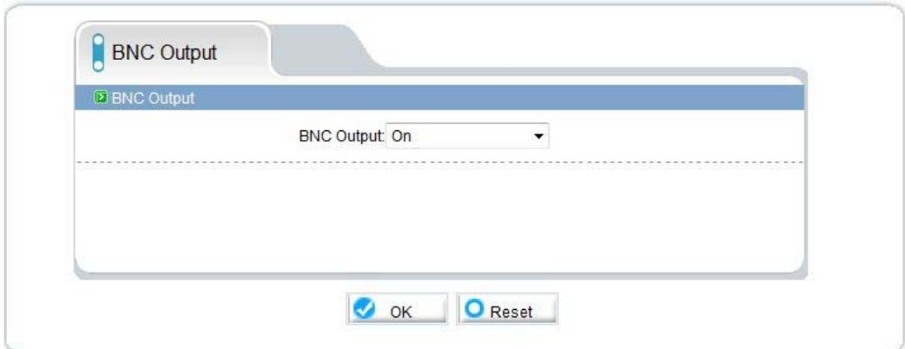
The RH Series cameras are equipped with BNC output that provides an analog composite video to connect a local monitor useful for example to adjust the camera lens in place without having to access the web via video. On this page you can enable or disable this output. If the BNC output is not used it is advisable to disable it in order to not unnecessarily CPU resources.
